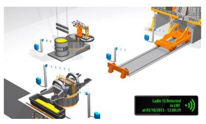
The system is distributed in different areas of the plant, and antennas are installed in specific spots where the ladles are to be detected. Each antenna will detect the RFID sensor installed on the ladles, and will communicate their location and unique information to the system Server via Ethernet.
