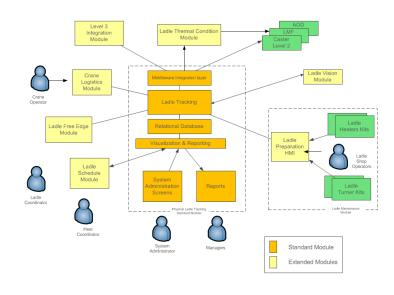
The PLT Framework takes care of configuration, rules and restrictions for the Meltshop operation, interacting as well with the supervised objects such as ladles and cranes, and their properties.
